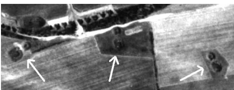
(Left) Figure 3. Light Flak battery at Einsatzhafen Rye, Gl. Ry Airfield Denmark November 6, 1941. The small dugout 'horseshoe' is the gun position, while the larger square one is the crew hut. The squares in the fields surrounding the positions mark the boundaries for the barbed wire fences
