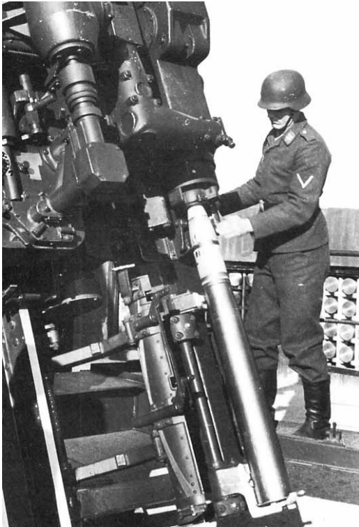
(Left) Figure 12. Automatic fuse setting before loading it into the chamber on a 12.8cm Flak. Note the stored ammunition in the back.
