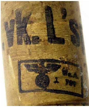
(Left) Figure 37: Work mark placed in a square on a 3.7cm shell. Note that a protective layer of weapon grease has been smeared on the entire shell/cartridge to protect it against moisture but at the same time making the colour look a bit darker. (The vk. on the shell before the L'spur (tracer) means Verkürzt – "shortened". It has a short burning tracer).
