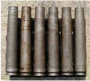
(Left) Figure 32: Steel 3.7cm Flak cartridges in matt light field grey colour, the brown stuff is not rust but weapon grease.
