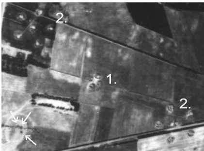
(Left) Figure 2. Two power, two predictor units (1.) and two six gun batteries (2.) situated in a heavy Flak battery at Fliiegerhorst Grove (today Karup Air Station) Denmark April 7, 1945. Note that the top positions are empty while the lower ones are occupied. However, they could easily be dummy guns. Also, note the three parked fighter aircraft in the lower left corner.
